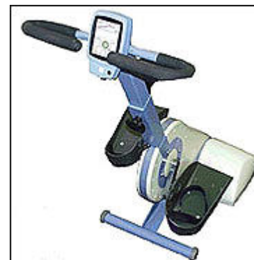
S6 Ergometer System consisting of a powered cycle, FES system, and PDA controller.
